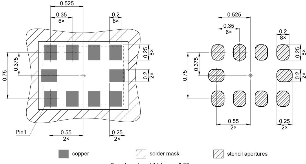
Based on stencil thickness: 0.08 mm
