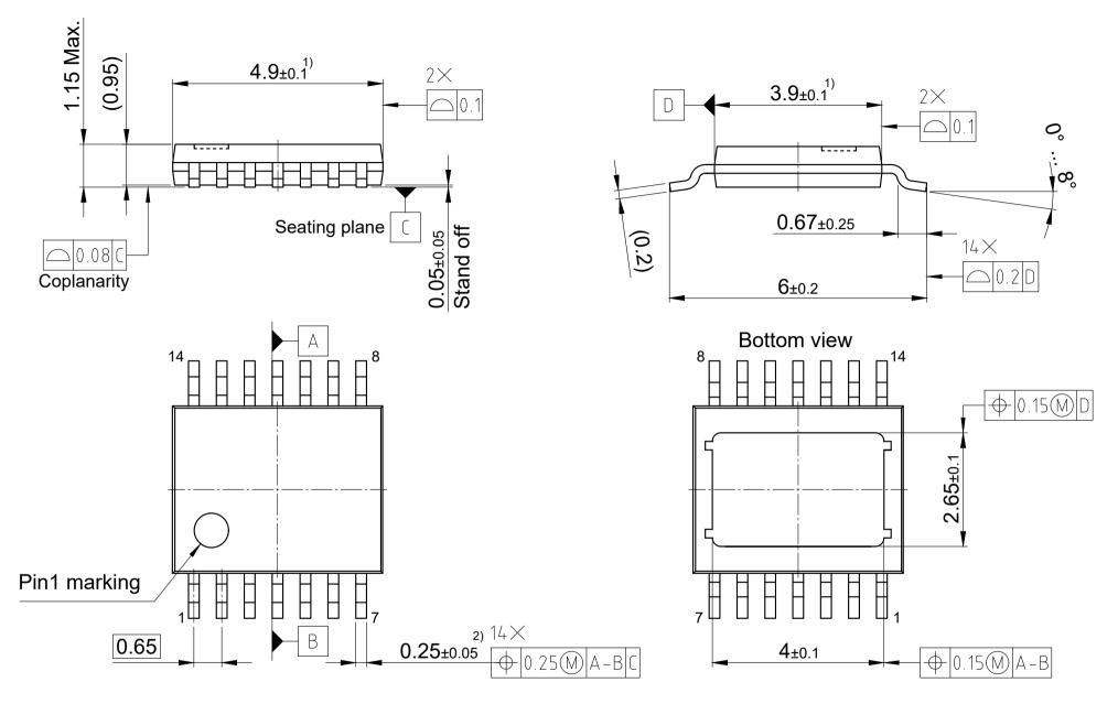
1) Does not include plastic or metal protrusion of 0.15 mm max. per side
