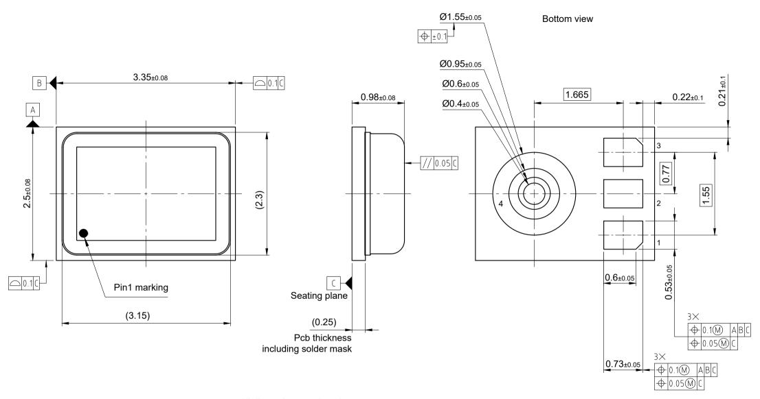
All dimensions are in units mm The drawing is in compliance with ISO 128-30, Projection Method 1 [ ] The drawing according to ISO 8015, general tolerances ISO 2768-mK
