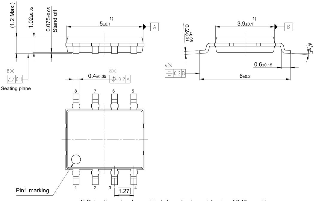
1) Outer dimension does not include protrusion or intrusion of 0.15 per side All dimensions are in units mm
