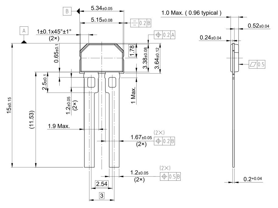
Outer dimension does not include protrusion or intrusion of 0.15 max. per side All dimensions are in units mm
