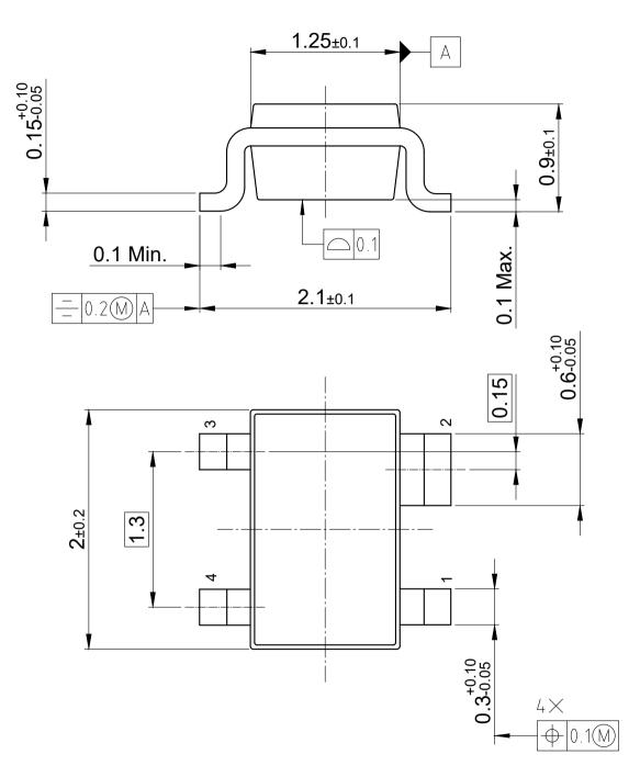
Mold flash, protrusions or gate burrs of 0.2 mm maximum per side are not include All dimensions are in units mm
