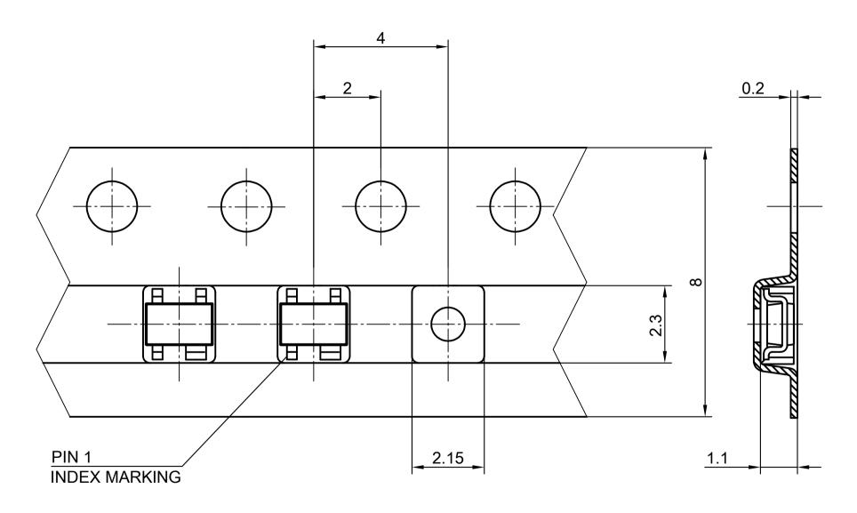
ALL DIMENSIONS ARE IN UNITS MM THE DRAWING IS IN COMPLIANCE WITH ISO 128 & PROJECTION METHOD 1 [  $\hfill \ensuremath{\bigcirc} \hfill \ens$
