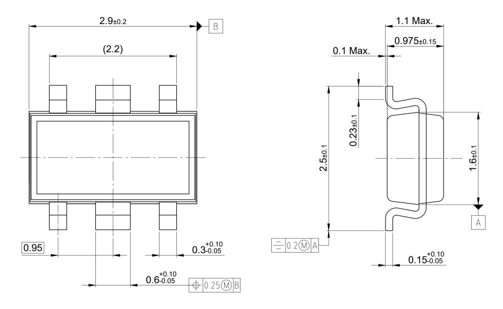
Note: Mold flash, protrusions or gate burrs of 0.2 mm maximum per side are not included All dimensions are in units mm
