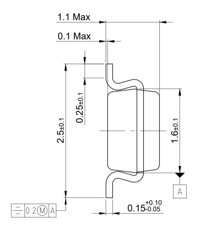
Note: Mold flash, protrusions or gate burrs of 0.2 mm maximum per side are not included
