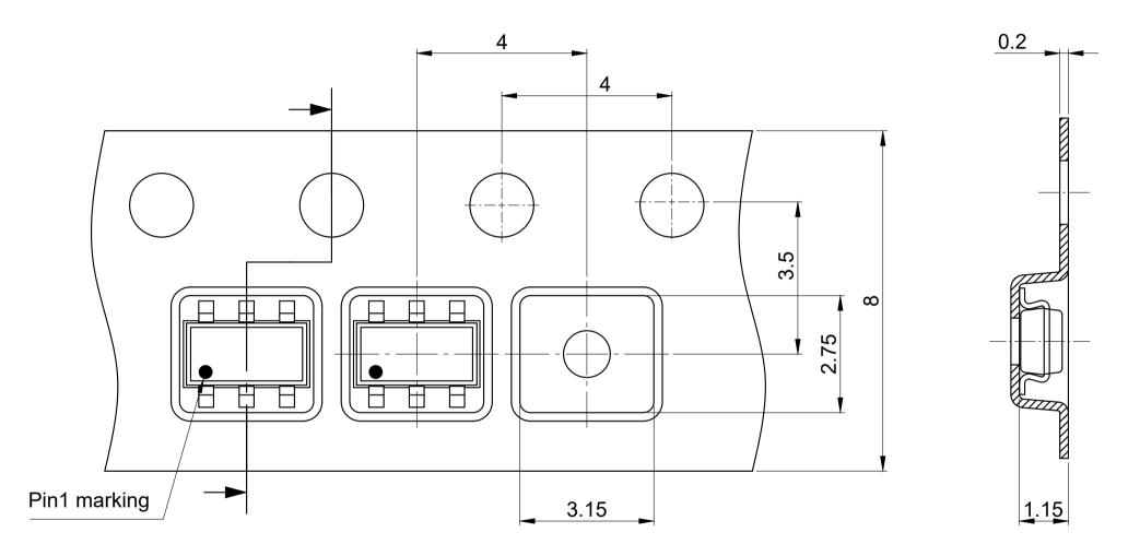
All dimensions are in units mm The drawing is in compliance with ISO 128-30, Projection Method 1 [  $\bigcirc$   $\bigcirc$  ]
