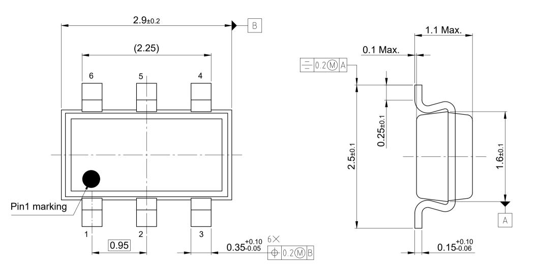
Note: Mold flash, protrusions or gate burrs of 0.2 mm maximum per side are not included All dimensions are in units mm The drawing is in compliance with ISO 128-30, Projection Method 1 [-]
