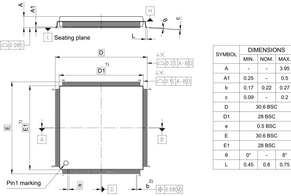
1) Dimensions D1 and E1 do not include mold protrusion.allowable protrusion is 0.25mm per side.
