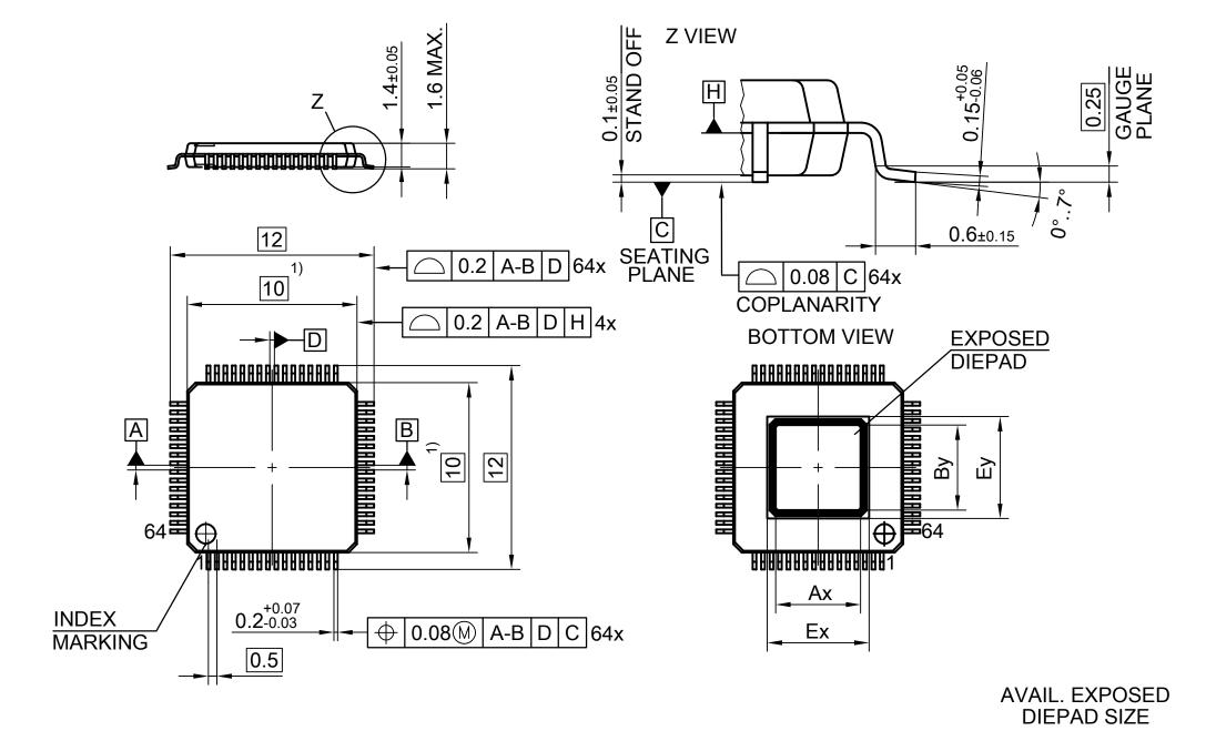
1) DOES NOT INCLUDE PLASTIC OR METAL PROTRUSION OF 0.25 MAX. PER SIDE ALL DIMENSIONS ARE IN UNITS MM
