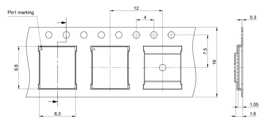
All dimensions are in units mm The drawing is in compliance with ISO 128-30, Projection Method 1 [ $\bigcirc \phi$ ]
