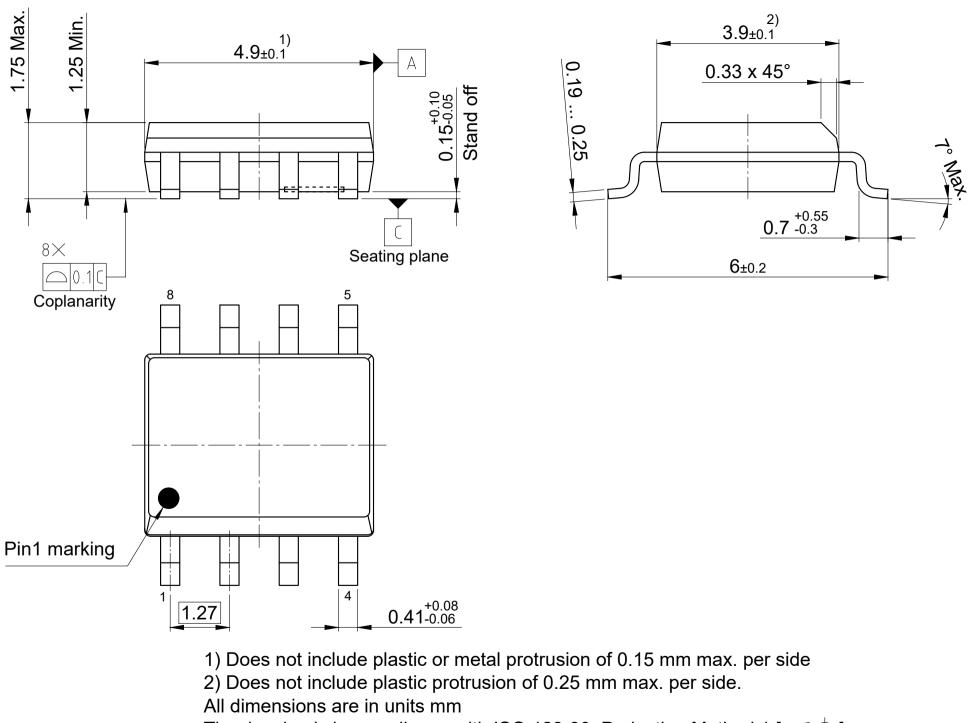
The drawing is in compliance with ISO 128-30, Projection Method 1 [ $\bigcirc$ ] Drawing according to ISO 8015, general tolerances ISO 2768-mK
