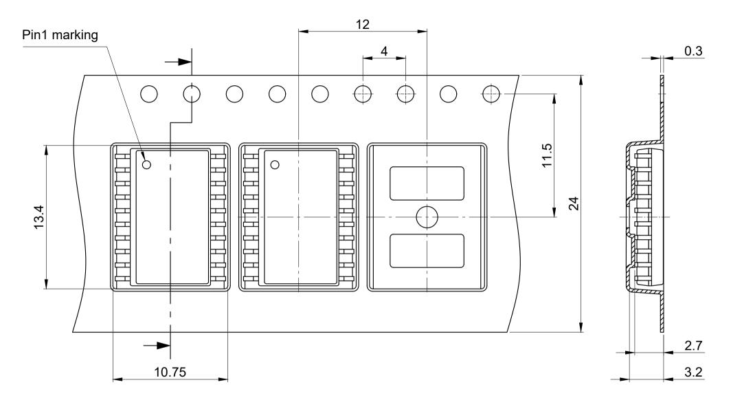
All dimensions are in units mm The drawing is in compliance with ISO 128-30, Projection Method 1 [ $\bigcirc \bigcirc$ ]
