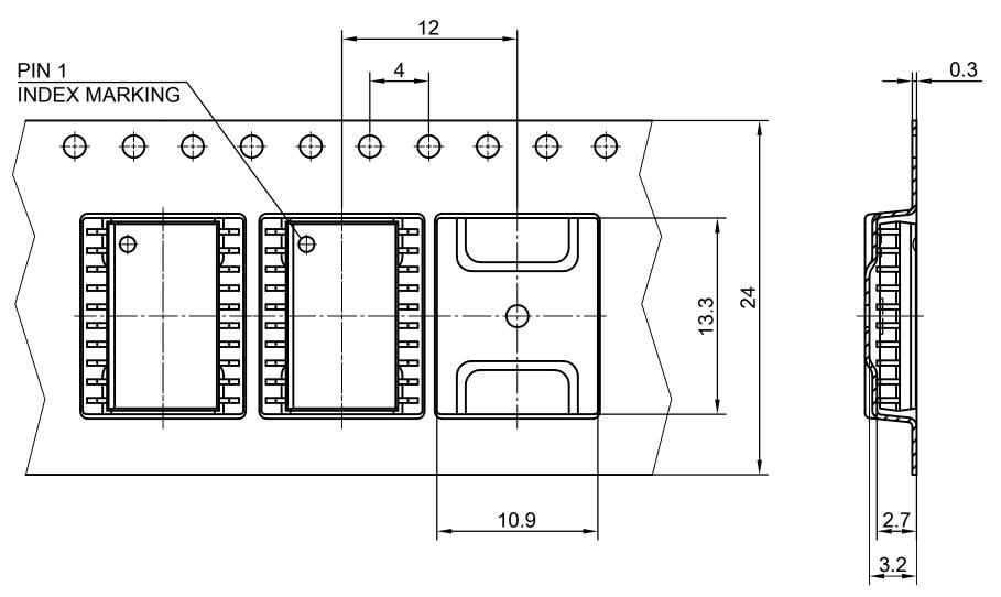
ALL DIMENSIONS ARE IN UNITS MM THE DRAWING IS IN COMPLIANCE WITH ISO 128 & PROJECTION METHOD 1 [  $\rightleftharpoons$  ]
