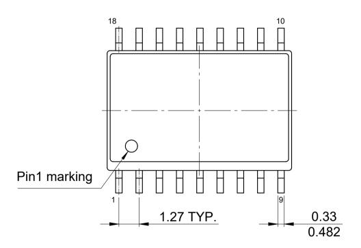
All dimensions are in units mm  $\frac{\text{min.}}{\text{max.}}$ The drawing is in compliance with ISO 128-30, Projection Method 1 [
