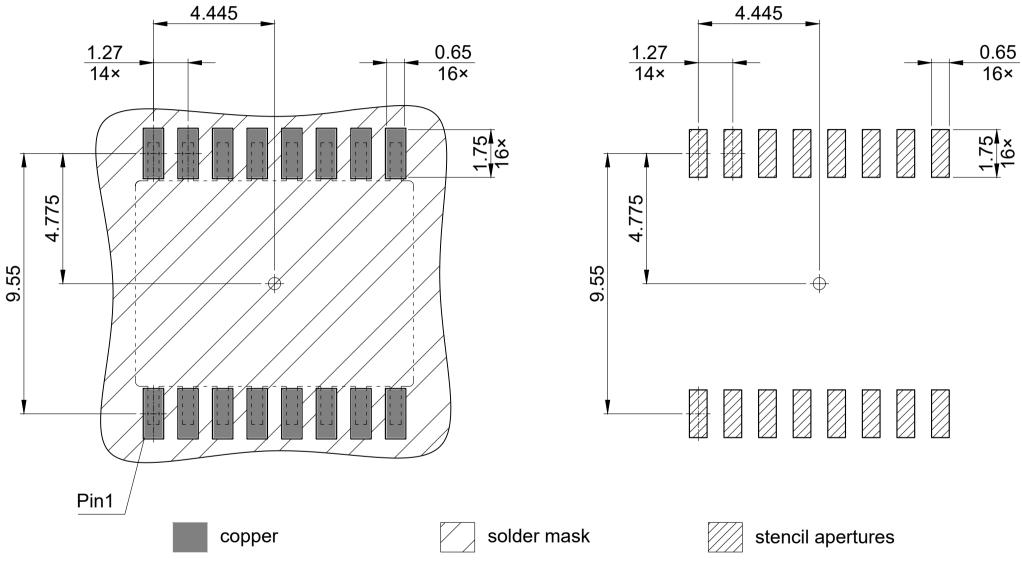
All pads are non-solder mask defined All dimensions are in units mm
