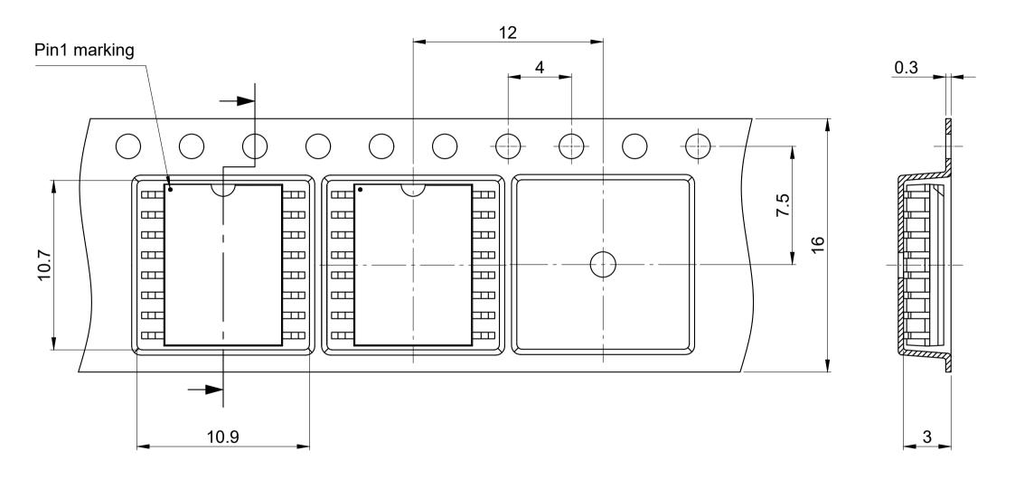
All dimensions are in units mm The drawing is in compliance with ISO 128-30, Projection Method 1 [ $\bigcirc \oplus$ ] Drawing according to ISO 8015, general tolerances MILLIMETERS
