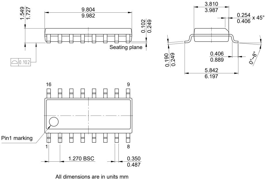
The drawing is in compliance with ISO 128-30, Projection Method 1 [ $\bigcirc \oplus$ ] Drawing according to ISO 8015, general tolerances ISO 2768-mK
