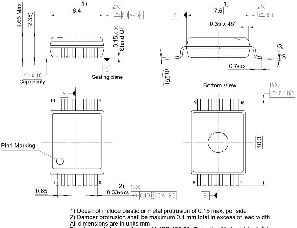
The drawing is in compliance with ISO 128-30, Projection Method 1 [ $\bigcirc \oplus$ ]
