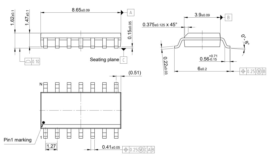
All dimensions are in units mm The drawing is in compliance with ISO 128-30, Projection Method 1 [-] Drawing according to ISO 8015, general tolerances ISO 2768-mK
