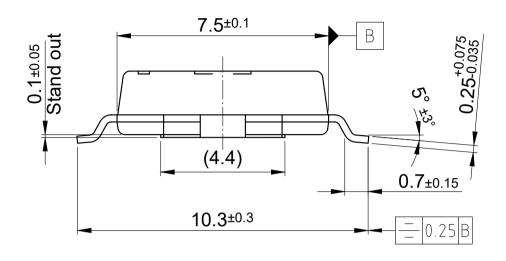
1) Does not include plastic or metal protrusion of 0.15 max. per side All dimensions are in units mm
