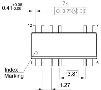
1) Does not include plastic or metal protrusion of 0.25 Max. per side
