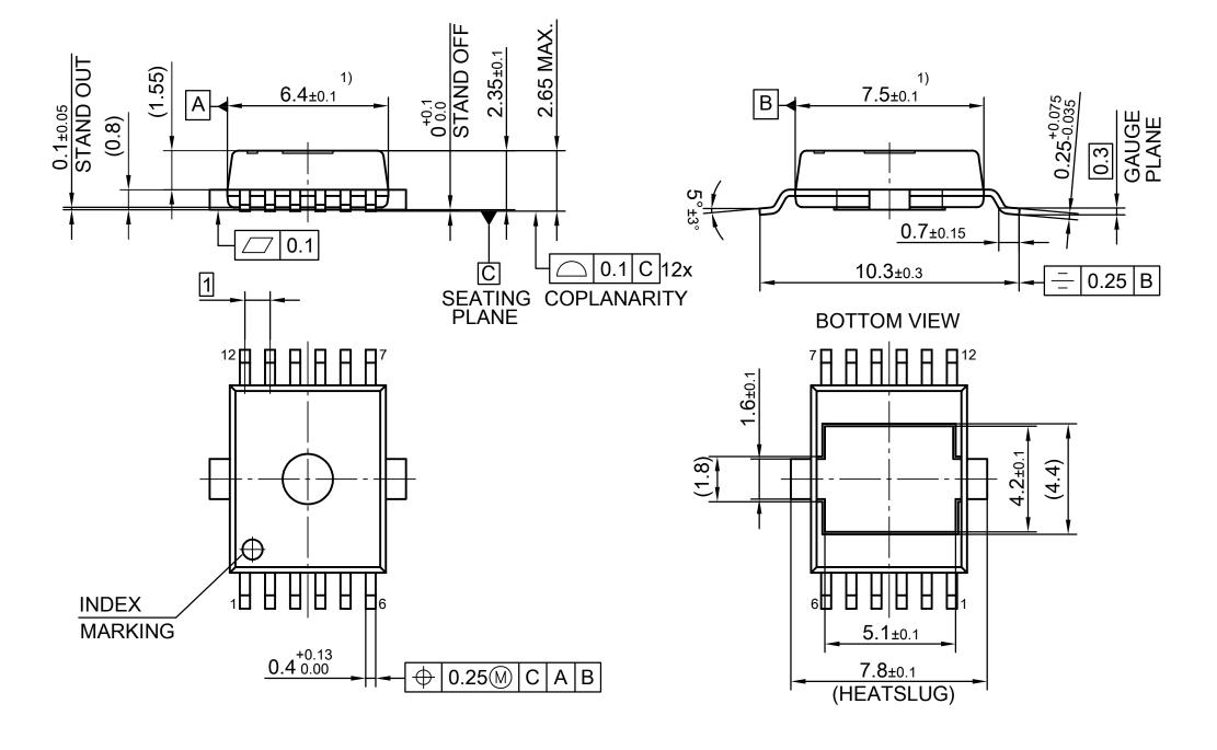
1) DOES NOT INCLUDE PLASTIC OR METAL PROTRUSION OF 0.15 MAX. PER SIDE ALL DIMENSIONS ARE IN UNITS MM
