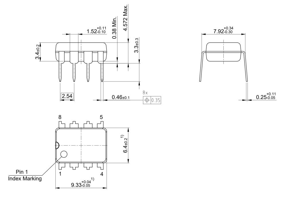
1) Does not include plastic or metal protrusion of 0.25 max. per side All dimensions are in units mm
