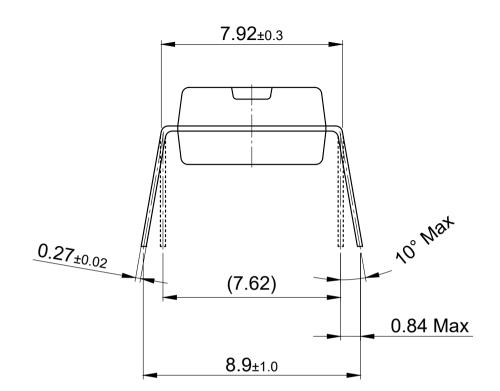
All dimensions are in units mm The drawing is in compliance with ISO 128-30, Projection Method 1 [ $\bigcirc \oplus$ ] Drawing according to ISO 8015, general tolerances ISO 2768-mK
