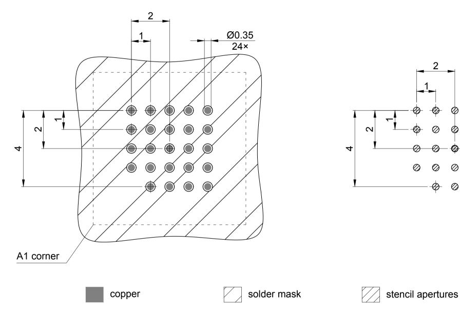
All dimensions are in units mm All pads are non-solder mask defined Ø0.35 24×
