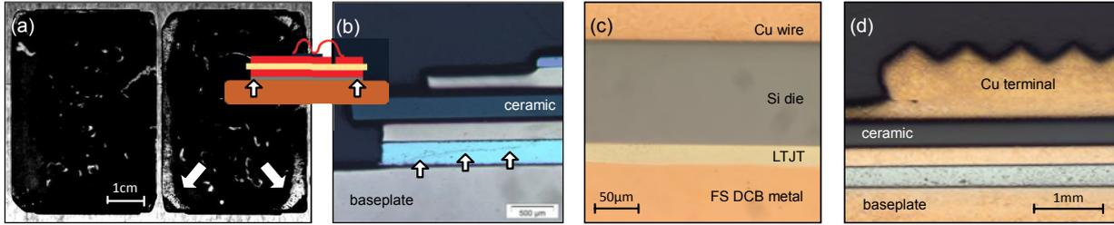
Fig. 11: .XT power module after 30kc  $PC_{min}$  with  $t_{on}=150sec$ ,  $dT=80K$  and  $T_{case,max}=105^{\circ}C$ . Acoustic microscopy image of substrate-baseplate interconnect (a) and cross-sections of substrate-baseplate joint (b), LTJT layer and top-side interconnect (c) and terminal (d).
