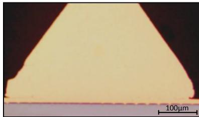
Fig. 1: Microsection of a Cu wedge bond on Si with Cu top-side metallization.
