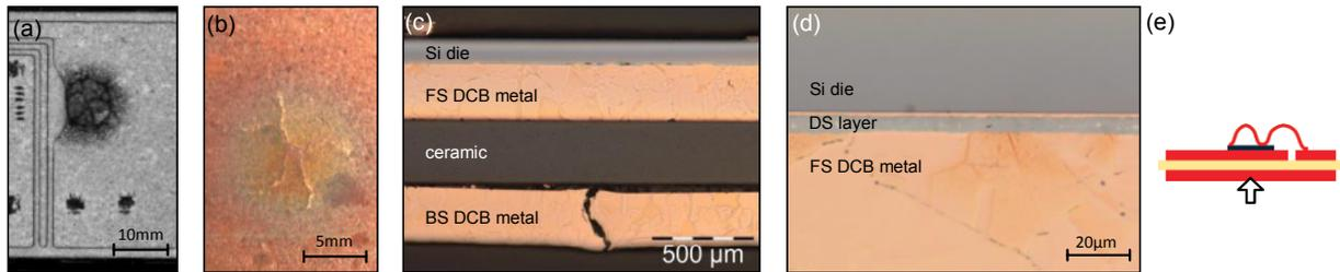
Fig. 7: .XT test sample with DS die attach w/o baseplate after 2.1mio short cycles at  $dT=107\text{K}$ . Acoustic image of the DCB interface (a), optical image of the DCB back-side (b), microsection of the test sample (c), the DS layer in detail (d) and location of major damage (e).
