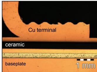
Fig. 5: Microsection of an ultrasonically (US) welded current terminal.
