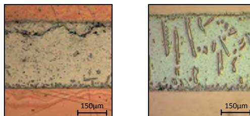
Fig. 4: Microsection of a standard Sn-Ag solder joint (left; after cyclic stress test) and a strengthened Sn based solder alloy.
