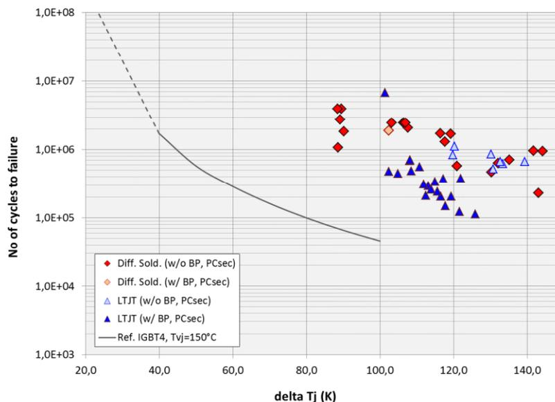
Fig. 6: Power cycling diagram for power modules w/ and w/o baseplates using .XT technologies. All samples use Cu wire bonding as top-side interconnect technology.
