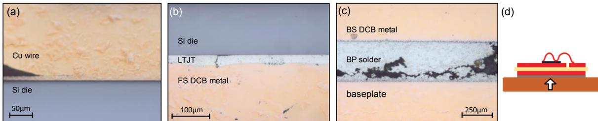
Fig. 10: Microsection of a test specimen w/ baseplate and LTJT die attach after 380k cycles PCsec with  $dT=122K$ . Detailed microsection of bond interconnect (a), LTJT interconnect (b), substrate-baseplate solder joint (c) and location of major damage (d).
