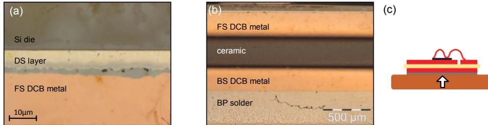
Fig. 9: Microsection of a test specimen w/ baseplate and DS die attach after 1.88mio cycles PCsec with  $dT=102K$ . Detailed microsection of DS layer (a), baseplate (BP) solder interconnect (b) and location of major damage (c).
