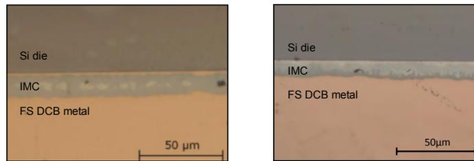
Fig. 2: Microsection of typical diffusion soldered die attach layers using Cu/Sn (left) and Ag/Sn (right) as intermetallic materials (IMC).
