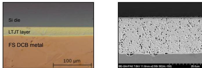
Fig. 3: Microsection of a sintered die attach layer with low porosity (left: optical, right: SEM).
