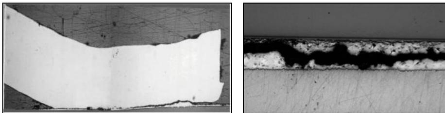
Fig. 1: Bond wire lift-off (left) and soft solder fatigue (right) after end-of-life power cycling with  $T_{j,max} = 150^\circ\text{C}$  using standard Al wire bonding and Sn based soft solders.
