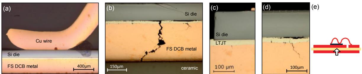
Fig. 8: .XT test sample with LTJT die attach w/o baseplate after 665k short cycles at  $dT=130\text{K}$ . Microsection of bond wire interconnect (a), fatigued area of substrate metallization (b), microsection of LTJT layer at edge (c) and at center (d) and location of major damage (e).
