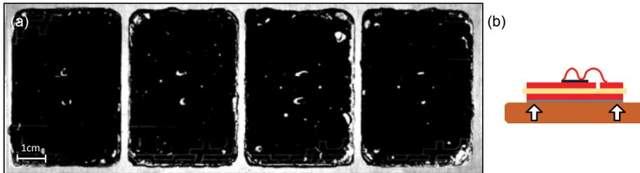
Fig. 12: Acoustic microscopy image of the .XT substrate-baseplate interconnect after 2000cycles TST ( $-40^{\circ}C - 150^{\circ}C$ ). Delaminated areas and voids are visible as white areas within the substrate region (a) and location of major damage (b).
