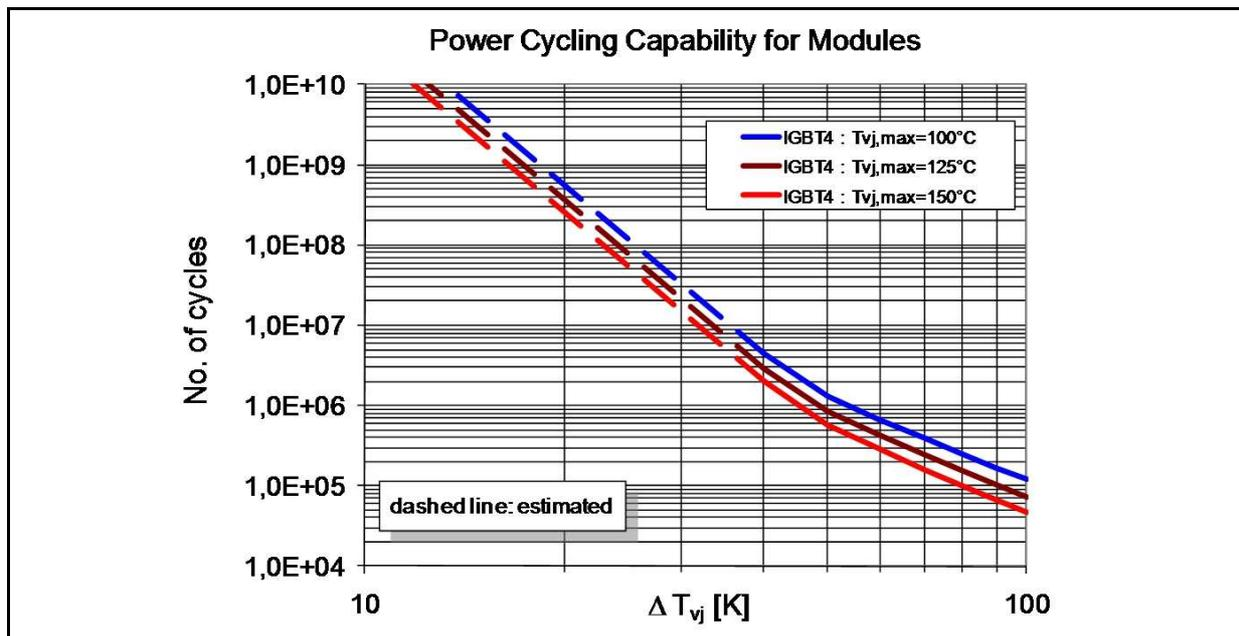
Figure 4: Power Cycling curve for industrial modules based on IGBT4
