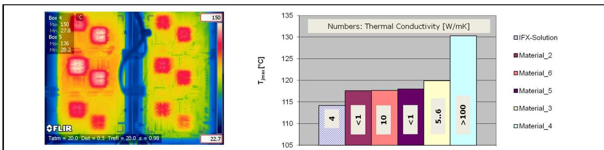
**Figure 2:** Thermographic measurement of chip temperatures using different thermal interfaces along with data gathered from six different materials
