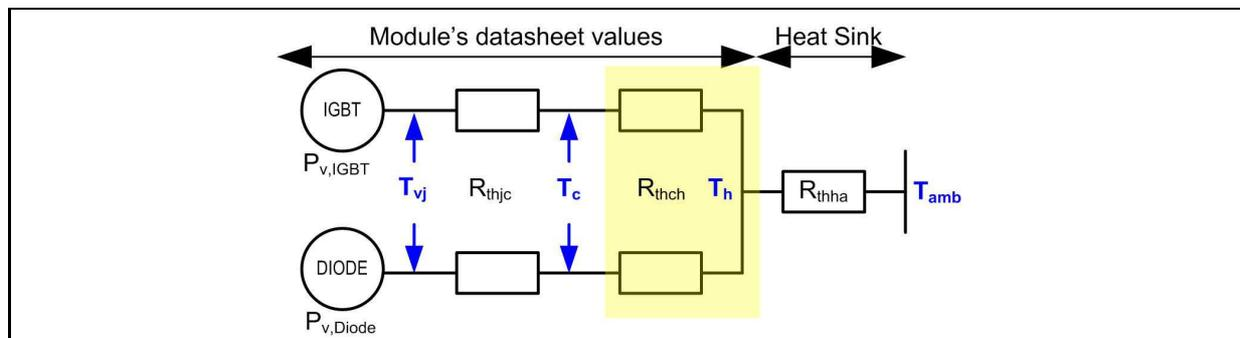
Figure 1: Simplified thermal model of a power electronic setup
