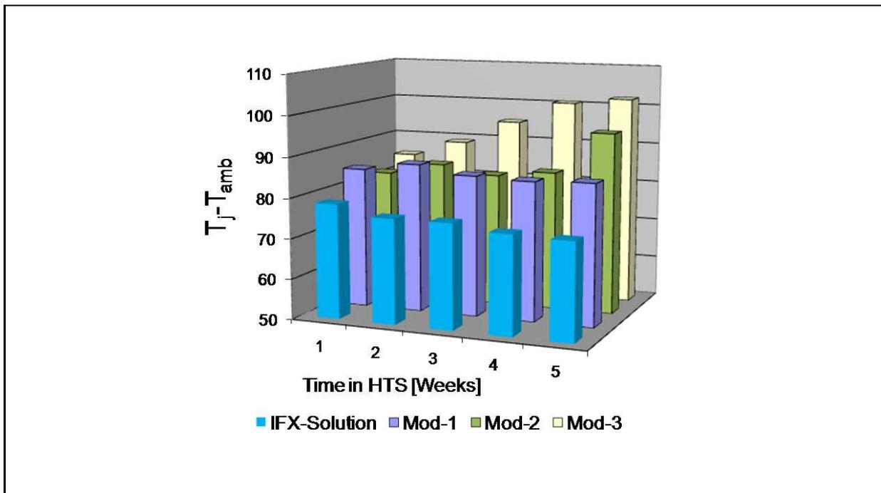
**Figure 3:** Thermal results from the 1000h HTS-Test
