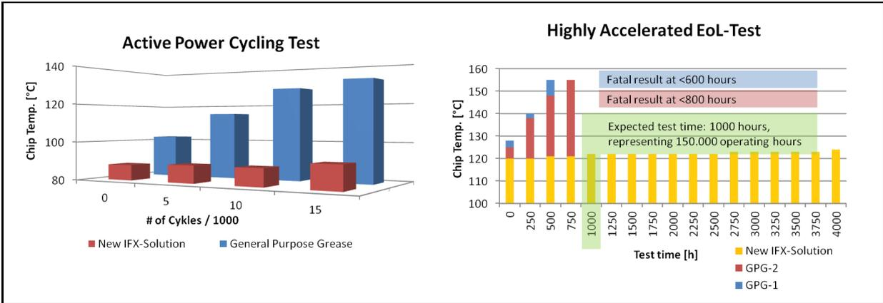
Figure 6: Results from Active Power Cycling to the left and HALT-Test to the right
