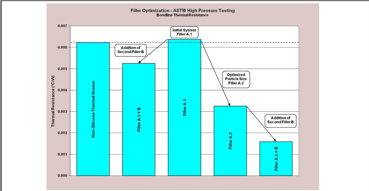
**Figure 3:** Evolution leading to the new solution using different material compositions, general purpose grease as a reference to the left
