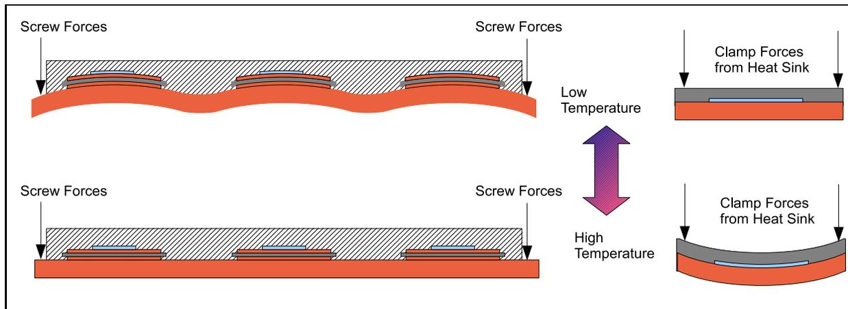
**Figure 2:** Comparison of thermo-mechanical movement in power electronic modules and discrete parts or CPUs
