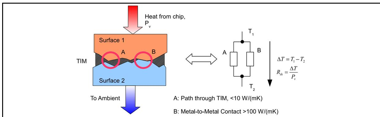
**Figure 1:** Microscopic view of thermal transfer paths connecting two different metallic materials
