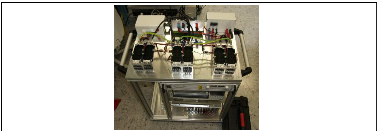
Figure 2: Test bench dedicated to conduct active thermal cycling featuring space to test six candidates at a time
