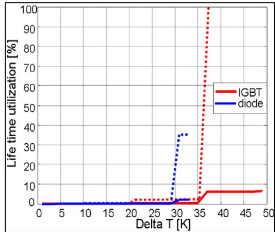
**Fig. 7.** Lifetime comparison of two modules. The dotted lines describe the utilization of the conventional technology. The IGBT with the standard technology defines the lifetime by reaching the 100 % limit. The continuous lines show the lifetime utilization of the .XT technology.
