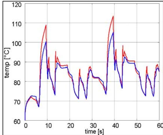
**Fig. 4.** Calculated junction temperatures of the IGBTs (red) and diodes (blue) based on the load profile.
