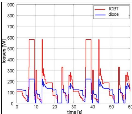
**Fig. 3.** Losses of the IGBT and the free wheeling diode
