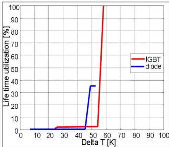
**Fig. 8.** Lifetime utilization of the FF900R12IP4LD with increased output current of 125% compared to the FF900R12IP4D after 25000h of operation.
