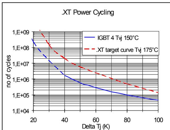
**Fig. 1.** PC diagram: Standard IGBT 4 Curve and IGBT4.XT power cycling limits for pulses with duration of about 1.5 seconds.
