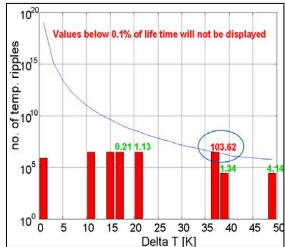
**Fig. 5.** Comparison of IGBT4 PC curve with needed lifetime of 25000 hours operation. The blue line is the PC curve. The red bars indicate the number of ripples for a temperature swing.
