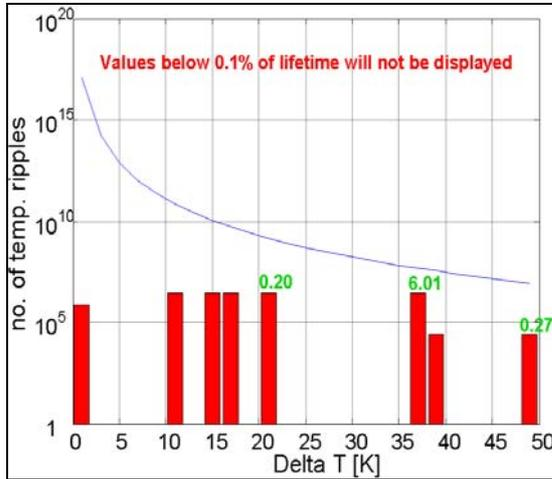
**Fig. 6.** Comparison of .XT power cycling curve with needed lifetime of 25000 hours operation
