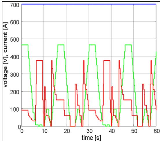
**Fig. 2.** Load profile with short pulses and high amplitudes. The blue line indicates the DC link voltage, whereas the green line is the voltage and the red line the current needed at the vehicles electric machine.
