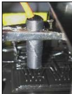
Fig. 9. IR- Sensor over covered IGBT chip
