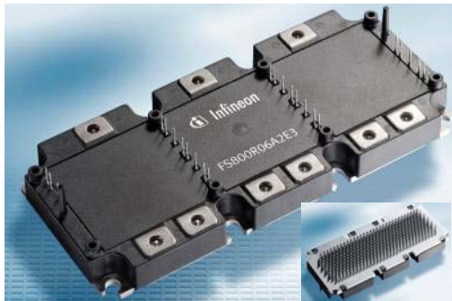
Fig. 5: investigated direct cooled HybridPACK 2 power module with Pin-Fin copper base plate
