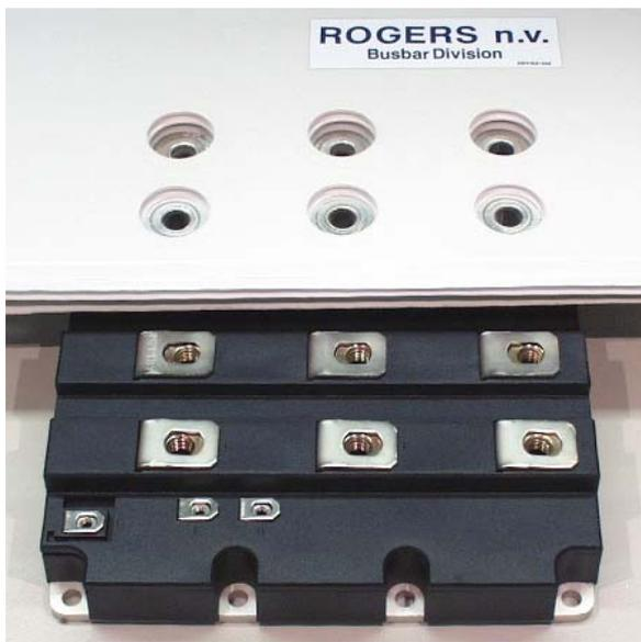
Figure 1: IHM A module and busbar
