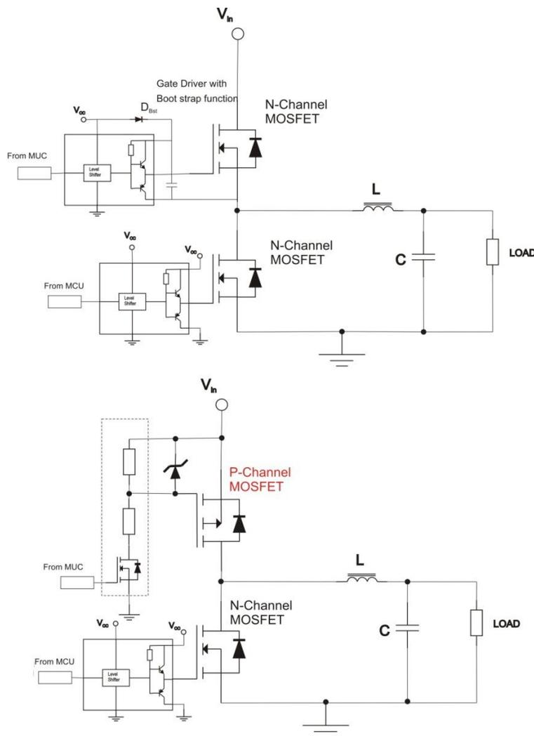
Figure 3.3: Buck converter circuit
