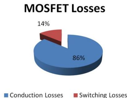
**Figure 3.2: MOSFET losses in the application**
