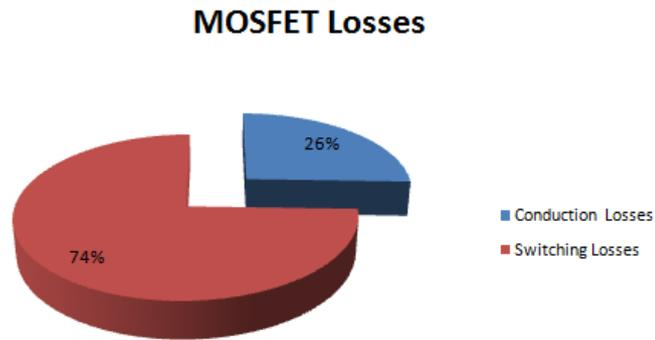
Figure 3.4: MOSFET losses in low power Buck Converters
