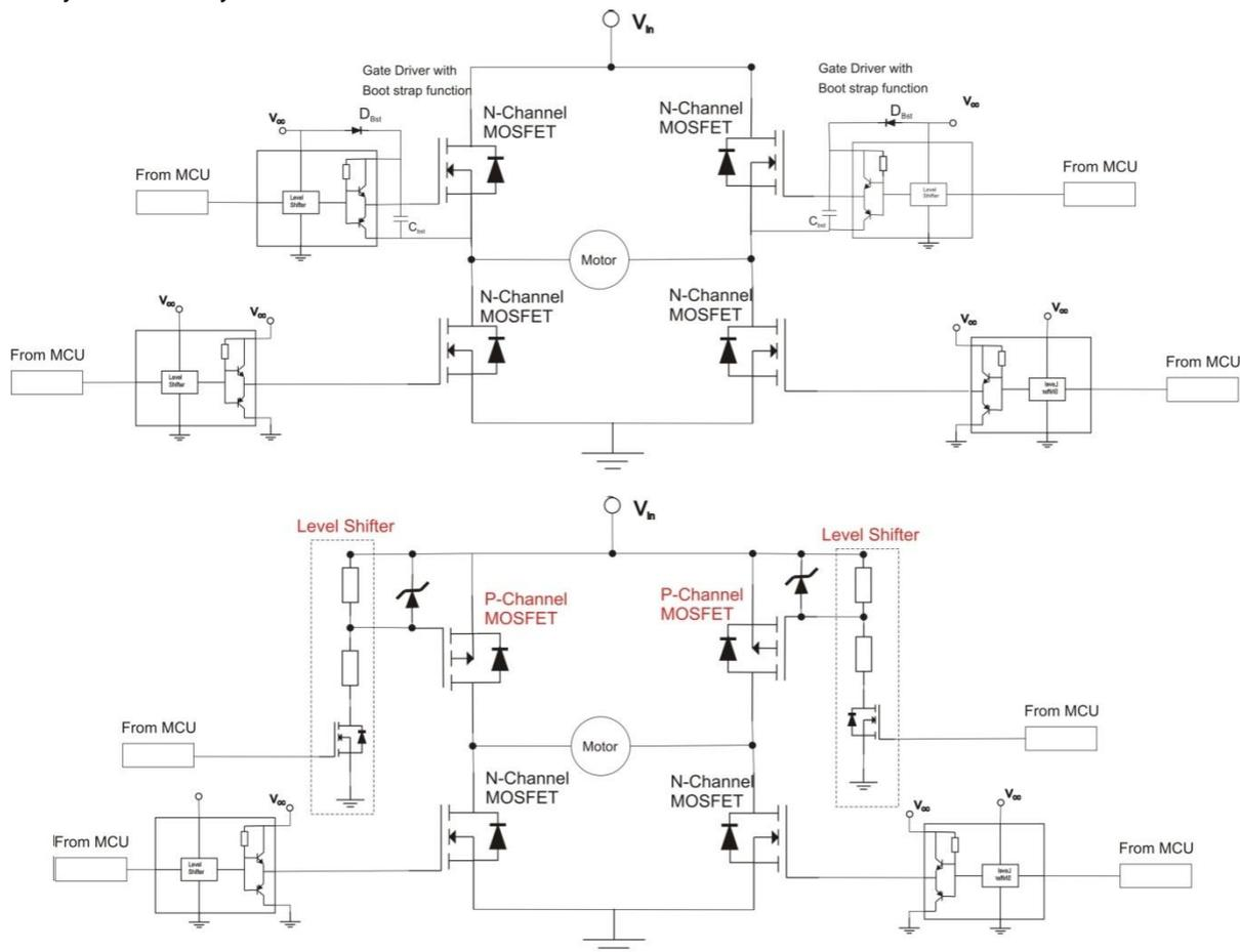
Figure 3.1: Low-Voltage drive application circuit
