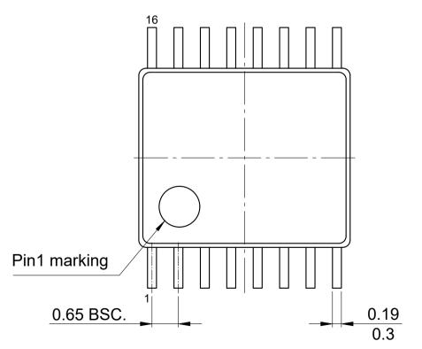
All dimensions are in units mm  $\frac{\text{min.}}{\text{max.}}$
