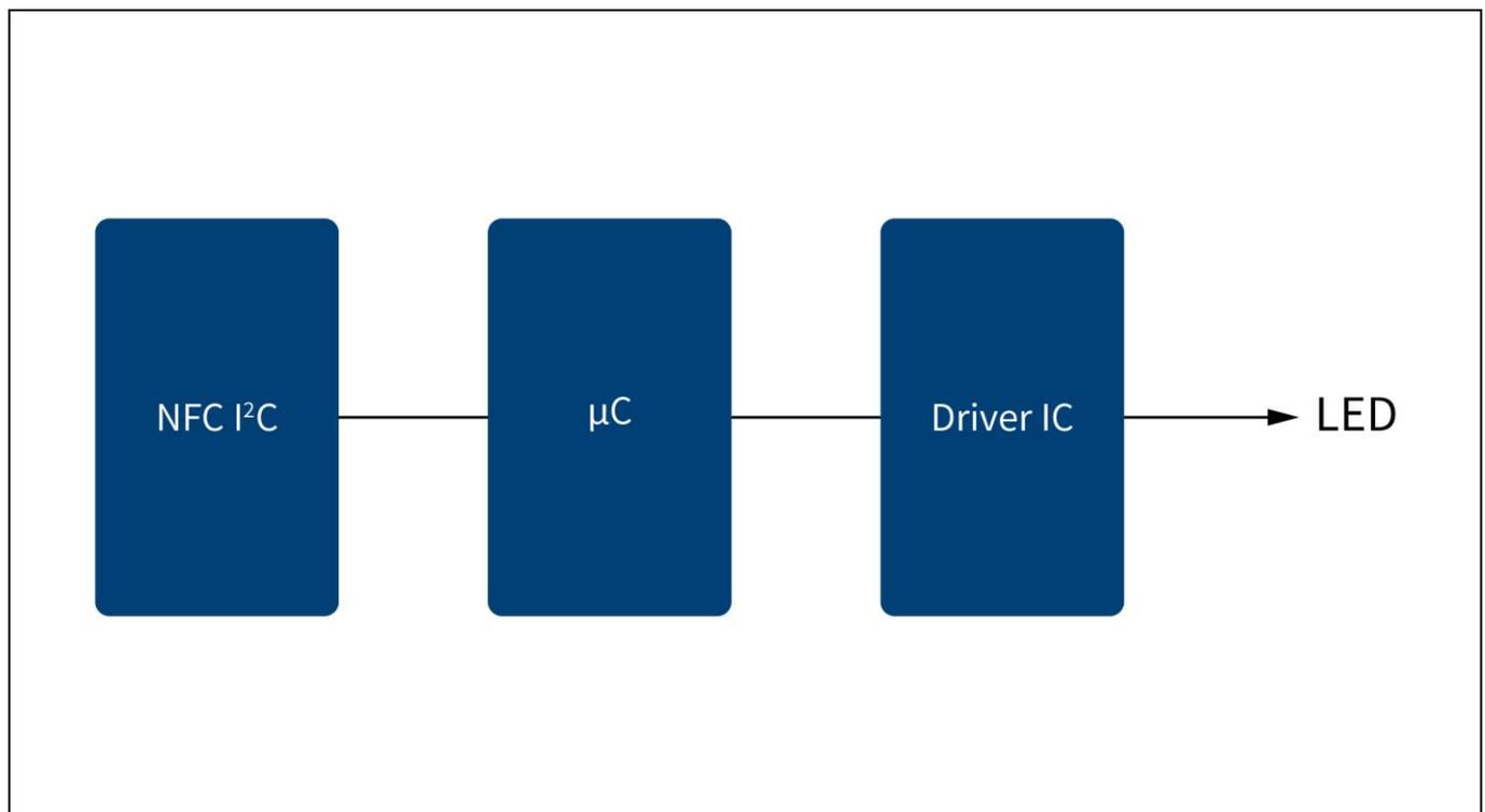
Figure 2 The traditional NFC-microcontroller concept
