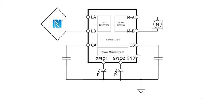
Figure 1 Smart Lock Example (Passive Supply Mode )
