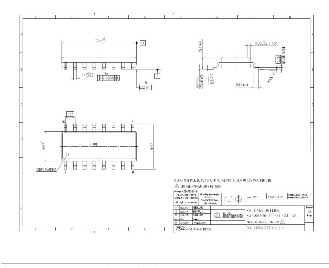
Figure 8 PG-DSO-16 Package Specification
