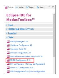
Similar to the make command method, launching the EZ-PD<sup>™</sup> Configurator using the Eclipse IDE opens the tool for the selected application. Refer to the <u>Eclipse IDE for ModusToolbox<sup>™</sup> user guide</u> for details about the IDE.
