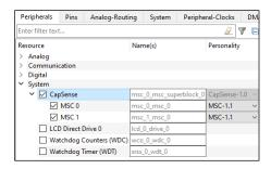
4. On the **Parameters** pane, click the **Launch CAPSENSE™ Configurator** button.
