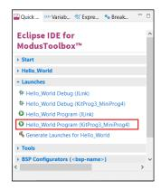
If needed, the IDE builds the application and messages display in the Console. If the build is successful, device programming starts immediately. If there are build errors, then error messages will indicate as such. When complete, the LED will start blinking.
