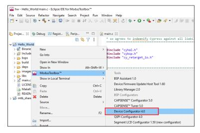
The Device Configurator provides access to the BSP resources and settings. Each enabled resource contains one or more links to the related API documentation. There are also buttons to open other configurators for CAPSENSE™, QSPI, Smart I/O, etc. For more information, refer to the <u>Device Configurator guide</u>, which is also available by selecting **View Help** from the tool's **Help** menu.
