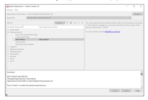
When the process completes, a message states that the application was created, and the Project Creator tool closes automatically. For more information, refer to the <u>Project Creator user guide</u>.
