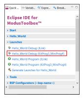
If needed, the IDE builds the application and messages display in the Console. If the build is successful, the IDE switches to debug mode automatically. If there are build errors, then error messages will indicate as such.
