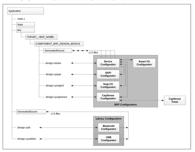
The following diagram shows a high-level view of the configurators in a typical application.
