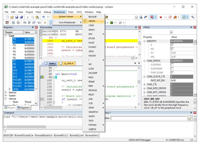
You can view the system and peripheral registers in the SVD view.
