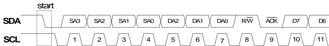
Figure 13-5. Addressing an I 2 C Peripheral
