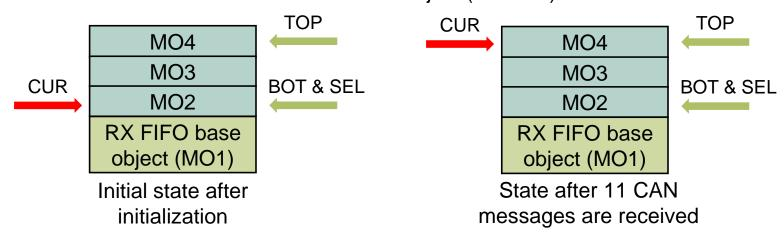
After 9 CAN messages are received, an overflow interrupt will be triggered and all the messages located in the RX FIFO object are read and stored in RX message structures. However, no additional overflow interrupt will be triggered after two additional CAN messages are received while the CUR pointer value is not equal to SEL pointer value. The additional CAN messages will be read by CPU only if any additional CAN message is received (CUR == SEL).
