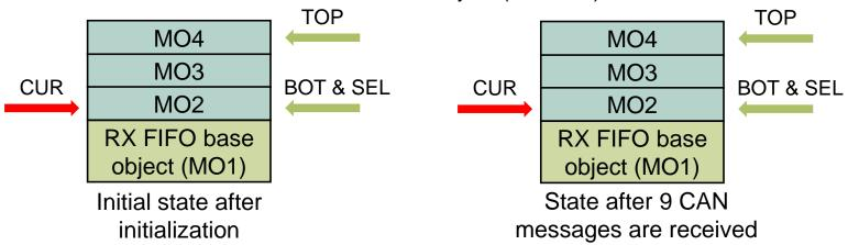
After 3 CAN messages are received, an overflow interrupt will be triggered (while the CUR pointer equals SEL pointer value) and all the messages located in the RX FIFO object are read and stored in RX message structures. After 6 and finally, after 9 CAN messages are received, same behavior can be observed.
