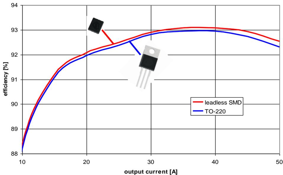
Figure 8: Experimental efficiency results for package comparison in a 12V SR stage
