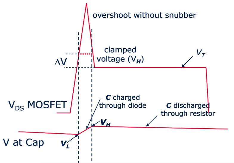
Figure 3: RCD snubber waveforms
