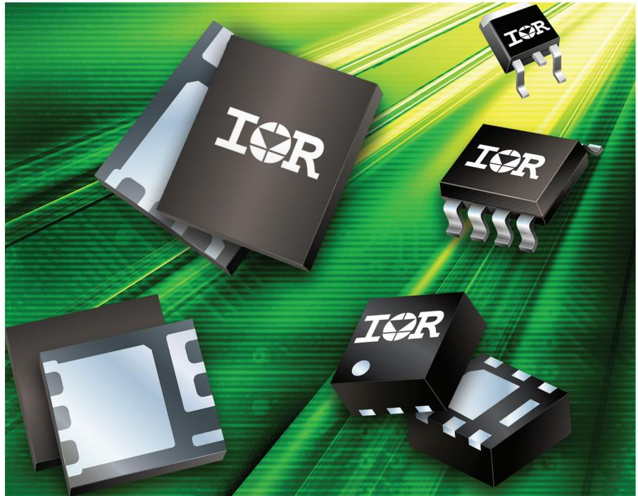
International Rectifier offers a series of 25V and 30V N-channel trench HEXFET® power MOSFETs featuring enhanced switching performance for synchronous buck converter and battery protection in computing applications for consumer and networking sectors.
