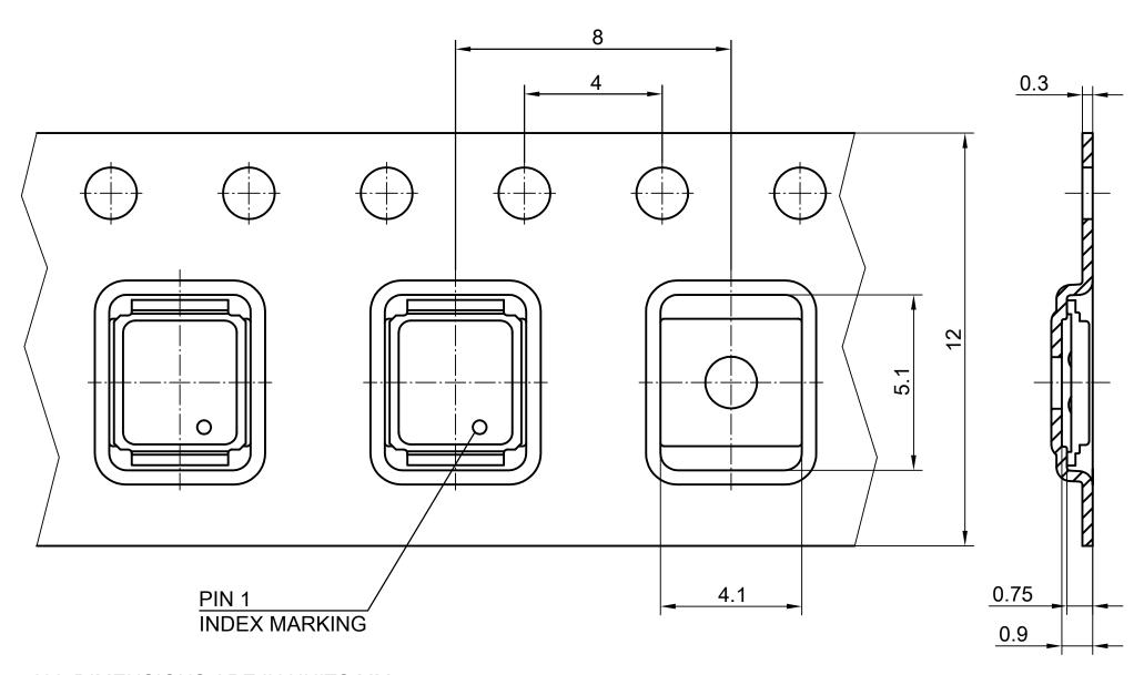
ALL DIMENSIONS ARE IN UNITS MM THE DRAWING IS IN COMPLIANCE WITH ISO 128 & PROJECTION METHOD 1 [  $\rightleftharpoons$  ]
